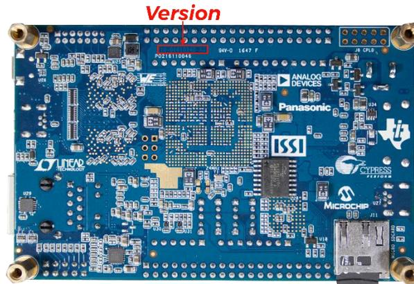
2. If there is an "A" printed at the specified location shown below, it refers to revision A. If the character is "B", it indicates the revision is B or B2. For revision C, the letter printed would be C.
